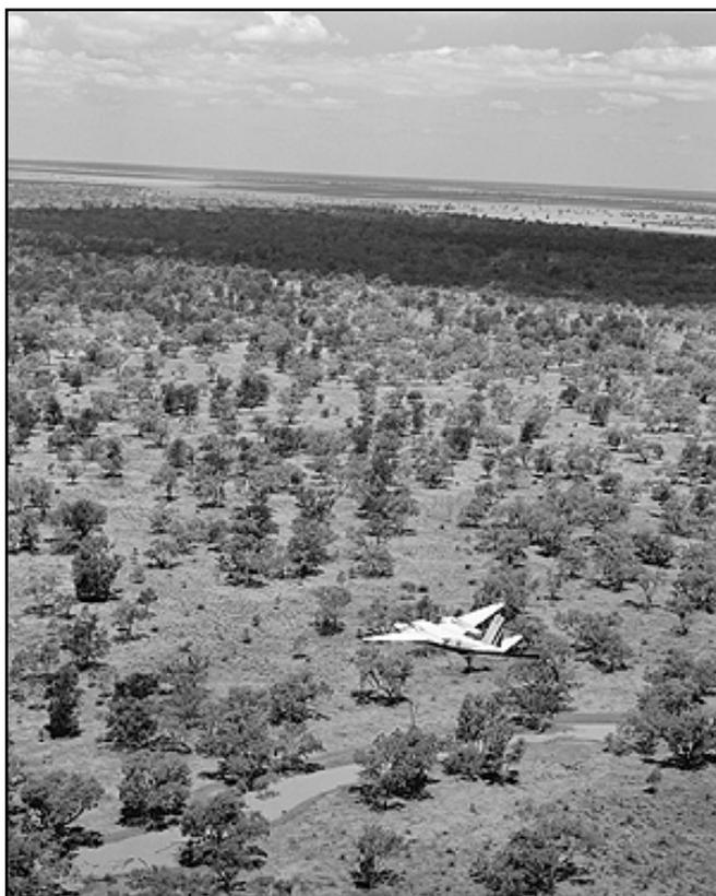
***Plane conducting aeromagnetic survey near Walgett - part of the recently completed 'Discovery 2000' exploration initiative. It is hoped that 'Discovery 2000' and its successor, 'Exploration NSW', will lead to the discovery of commercial petroleum deposits in NSW***
